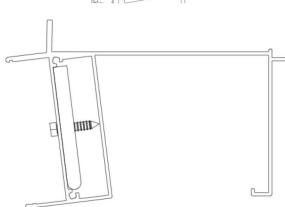
Fix the steel bar into position with drill screws no more than 20mm in length
