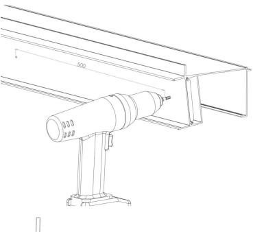
Pre-drill a 3mm hole through the back of the gutter into the steel bar at approx. 500mm intervals along the length of the gutter. Be careful not to pierce the inside wall of the gutter.
